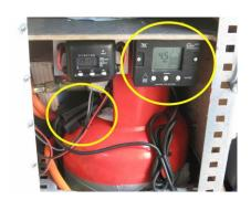
Nevertheless, gas under pressure can be sneaky. Through constant vibration on rough roads it is not impossible that a tube might become chafed, a valve becomes loose or gas escapes by other means. As a precaution measure, I always have the main valve closed when driving. In addition, I have installed a gas alarm that makes me aware of any leakage.
