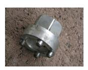
The second protection I have are coded screw nuts to prevent theft of my wheels. I replaced one of the standard nuts with this special nut on each wheel. They can only be unscrewed with a special (coded) adapter. Five such nuts cost me 140 CHF and I think the invesment is worth it. However, pay attention where you keep the adapter in case you have todo a wheel change. And don't loose it either.
